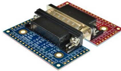
Figure 4: Solid Male to Female connection with the 4-40UNC diameter 8.3mm long screws
