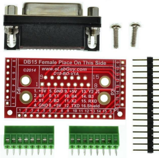
Figure 1: Parts inside the kit (Note: the module is not assembled, user can decide which connector to use on the module.)
